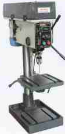
Drilling & Tapping Machine with Variable Frequency Drive (VFD)
